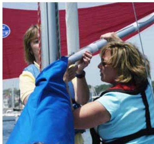
*Attaching the spinnaker pole to the mast.*
